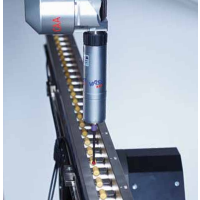
Test of length measurement error E0 with a step gauge in space.
