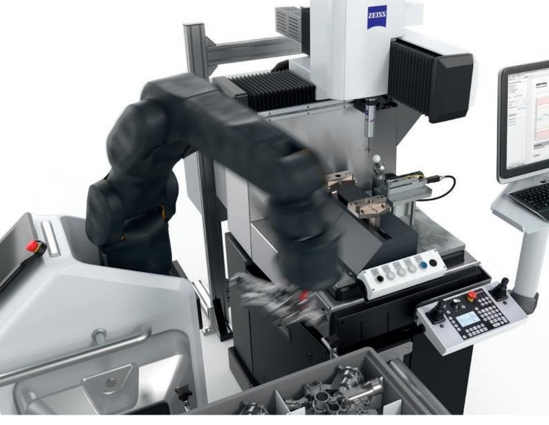
The flexible measurement system, consisting of a collaborative robot and a ZEISS DuraMax HTG, reduces the metrology engineer's day-to-day workload while simultaneously increasing productivity.
