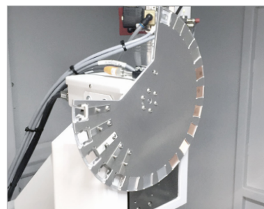
An automated filter wheel installed on the ZEISS METROTOM 800.
