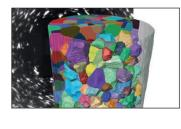
Analysis of grain size & distribution Grain size and distribution are decisive factors in determining the hardness and strength. This is why it is important to analyze them.
