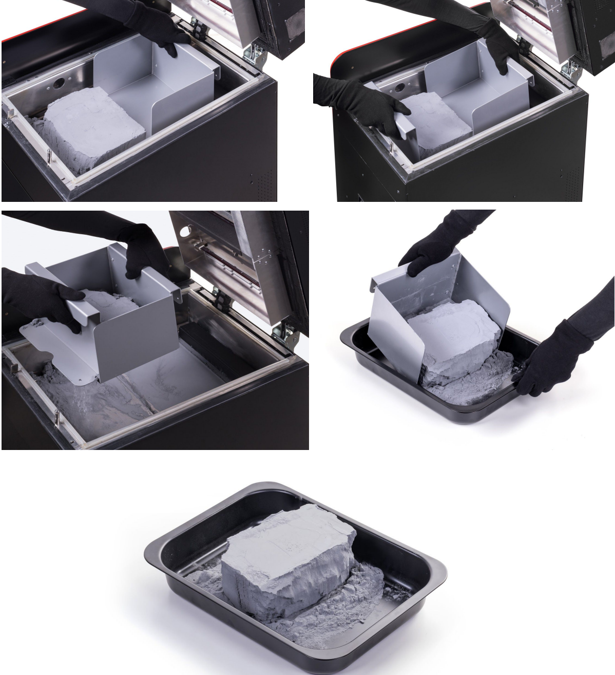
Image. A correct way of taking out the prints from the Print Bed
