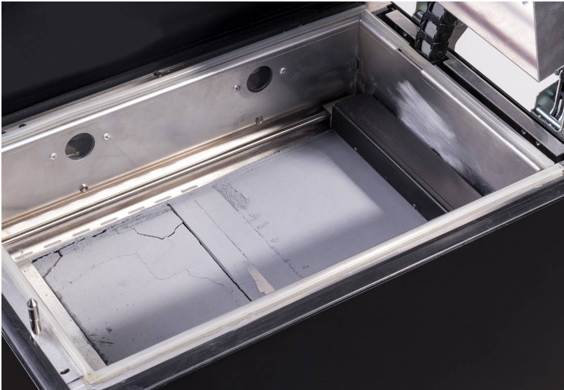
Image. A correct condition of the powder after printing (visible cracks on the surfaces of both Beds).
