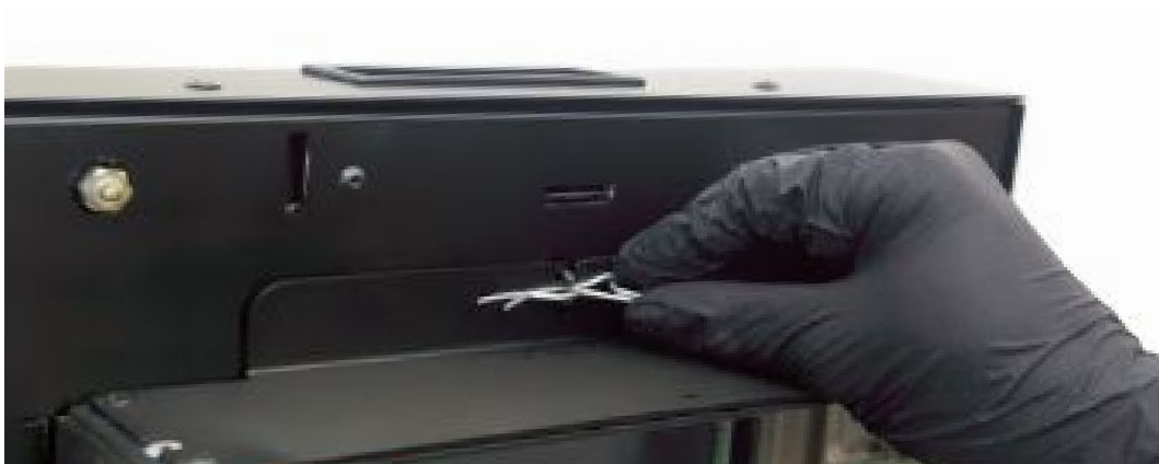
Image. heater module - split pin system
