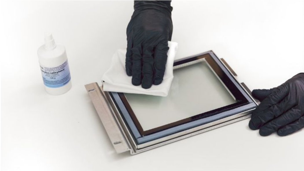
Image. Cleaning of laser protection glass
