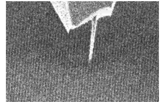
FIB sharpened AFM tip for high aspect ratio measurements.
