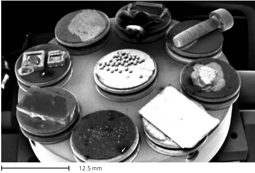
Figure 1 Nine way carousel holder with 12.5 mm diameter stubs
