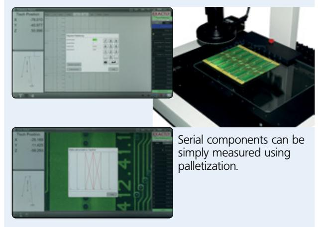
Serial components can be simply measured using palletization.
