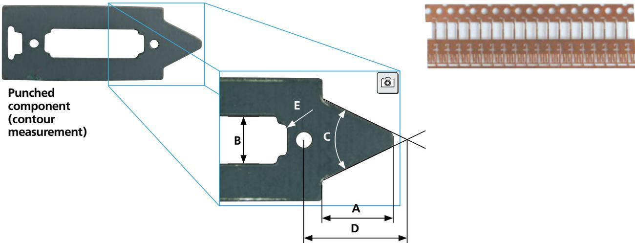
Punched component (contour measurement)
