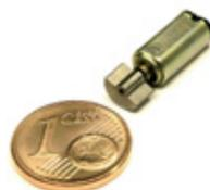
Vibrating motor for a mobile phone
